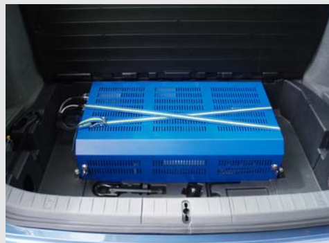
Main on-board electronics housed in the boot
